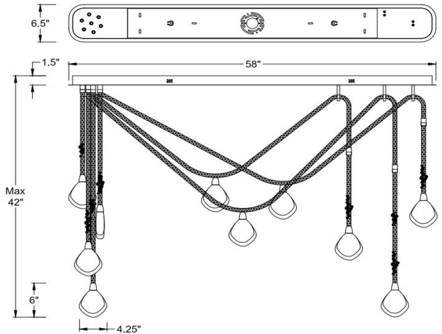
Fixtures weighing 35 lbs. or more must be supported and installed independently of the ceiling outlet (junction) box and require additional support in the ceiling where the fixture is being installed
